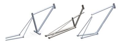
**FIGURE 4**: Examples of geometrically infeasible bicycle frame models from the FRAMED dataset.
