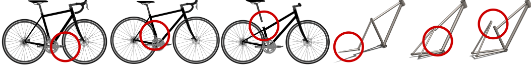
Figure 10: BikeBench features numerous closed-form constraint checks to identify common geometric infeasibilities such as disconnected or colliding components (left 3). Less common infeasibilities in frame geometry are flagged if the design causes errors during 3D reconstruction (right 3).
